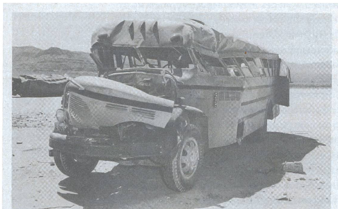
Figure 5.96c. Typical public bus damaged by a nuclear explosion, Nevada Test Site; this bus, like the one in the left background, was overturned, coming to rest as shown after a displacement of 50 feet.
