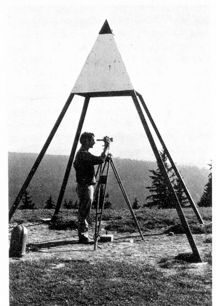
Measuring vertical angles with a theodolite
