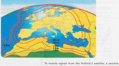
dish at least 60 cm in diameter, which is equipped for digital broadcasting, plus a universal LNB (Low Noise Bloc, resize of satellite dish you'll need in your region.
