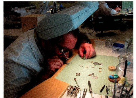
Workbenches, made locally, are modeled after the traditional watchmaker's bench in Switzerland, with indented arm rests that help keep the watchmaker's hands steady.
