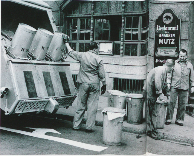
In 1897, the Zurich engineer Jakob Ochsner developed a dust-free waste disposal system and later on the legendary rubbish bin
