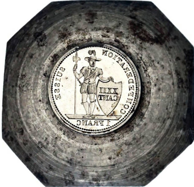
A die for the screw-press striking of the one franc coin showing a coat of arms. Canton of Vaud, Lausanne, 1846.
