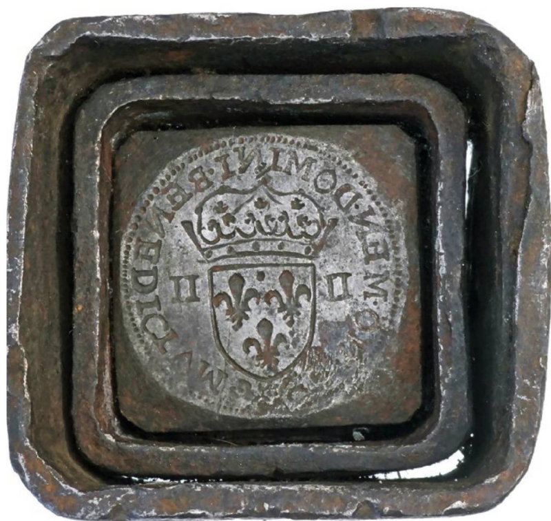
A moveable iron die for the falling-hammer or screw-press striking of the quarter ecu coin. Kingdom of France, Henry IV (1589 to 1610), unknown mint.
