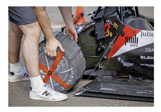
ABOVE: Putting on warm tyres. The suction device is visible close to the ground.
