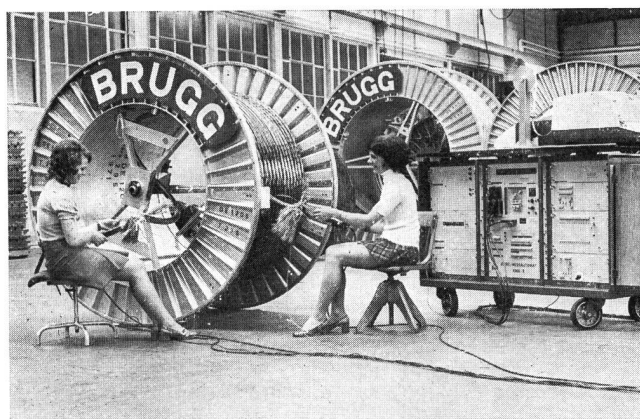
Fig. 4 Operators testing a factory length of cable by means of automatic tester KMA-3b
