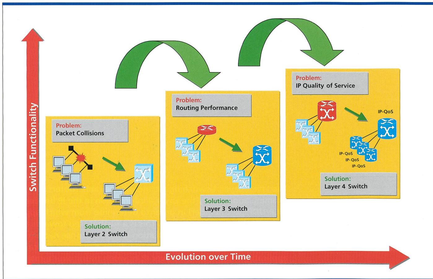
Fig. 1. Evolution from Layer 2 towards Layer 4 switches.
