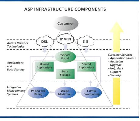
The figure presents an overview of the components of the ASP infrastructure. It shows how the customer is provided with applications and service through the access network, applications and data storage and integrated management systems layers. The customer services depend on all three layers; the end-user makes use of an application hosted in the data centre through the access network and is correctly billed for that usage because of the usage mediation, pricing and billing management systems.
