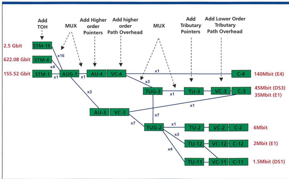
Bild 1. SDH-Multiplexing-Hierarchie für STM-1 (SDH: Synchronous Data Hierarchy, STM: Synchronous Transfer Mode, AUG: Administrative Unit Group, AU: Administrative Unit, VC: Virtual Container, TUG: Tributary Unit Group, TU: Tributary Unit, C: Container).
