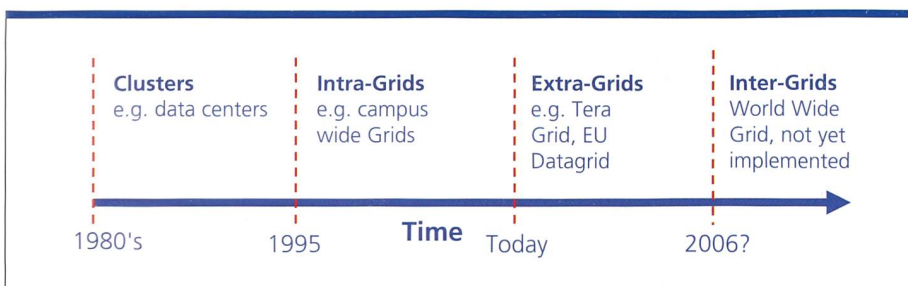
Fig. 4. Grid topologies evolution.
