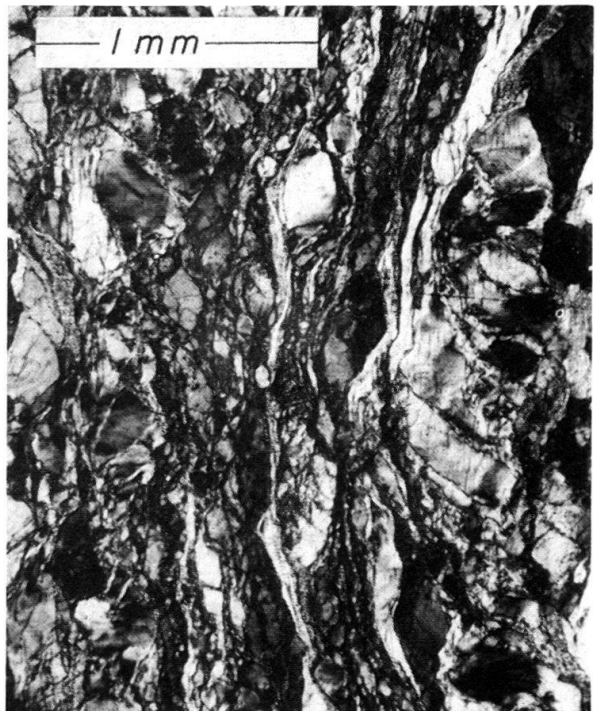
Fig. 12. Photomicrographs of mylonitic rocks close to the granite contact (1 km). a) Sci 308. Bergell granite N P. Cengalo. b) Sci 535. Tambo gneiss, V. Torta, 1,070 m, S. Vicosoprano. c) Sci 216. Gruf migmatite, Btta. Tegiola. d) VW 35. Experimentally deformed Cathedral peak quartz monzonite (compare Fig. 11a). Conditions: 900°C, 15kb confining pressure, 10^{-6} sec ^{-1} strain-rate, 60% shortening.
