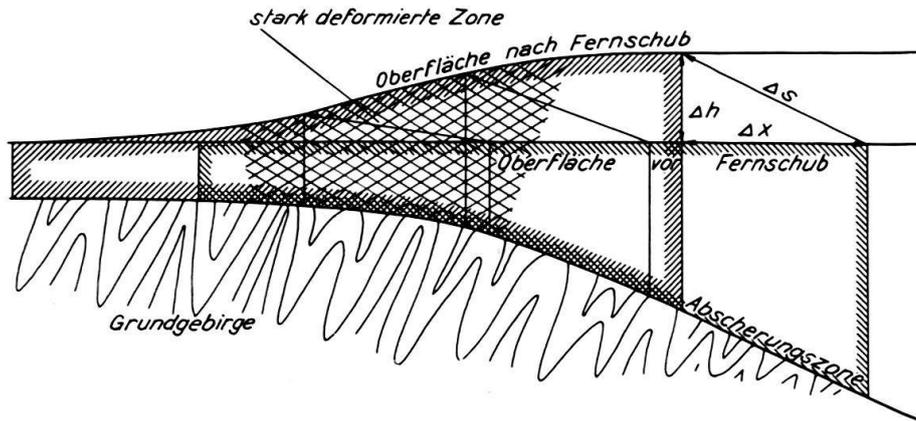
Fig. 1. Surface uplift above a stationary basement, due to decollement (uphill translation of a sedimentary wedge). From LAUBSCHER (1961).
