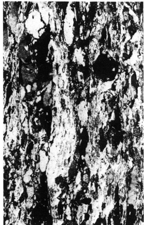
Fig. 5. Optical micrograph of the ultramylonitic handspecimen (No. 3 in Figure 3). Leucocratic bands consist of quartz and albite, melanocratic laminae consist of white mica and epidote. A hypidiomorphic garnet is seen in the upper right-hand corner. Height of photograph 0.6 mm, crossed polarizers.
