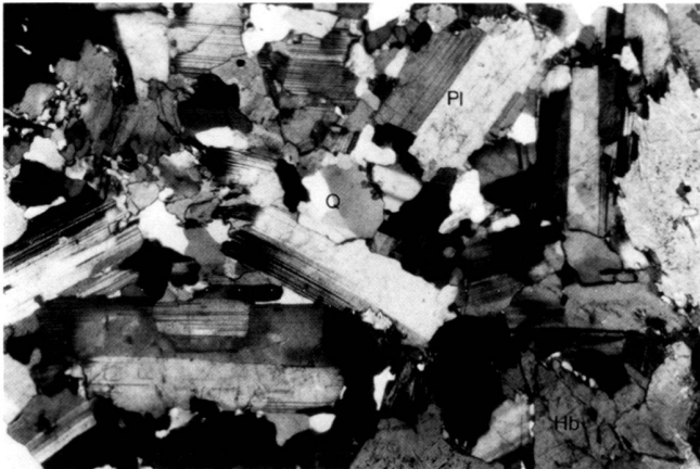
Fig. 4. Thin section of tonalite from Site 2. Longer sides of picture are 5 mm. No shape preferred orientation nor plastic deformation are present within this sample. Q: quartz, Hb: hornblende, Pl: plagioclase.
