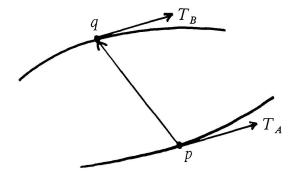
where e is a direction vector between two points, p and q, one from each curve.  $T_A$  and  $T_B$  are unit tangent vectors to the curves at these points.
