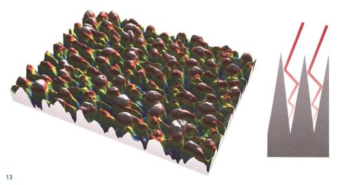
13 With increasing energy, the ripples are gradually transformed into spikes, very small and narrow pyramids.
