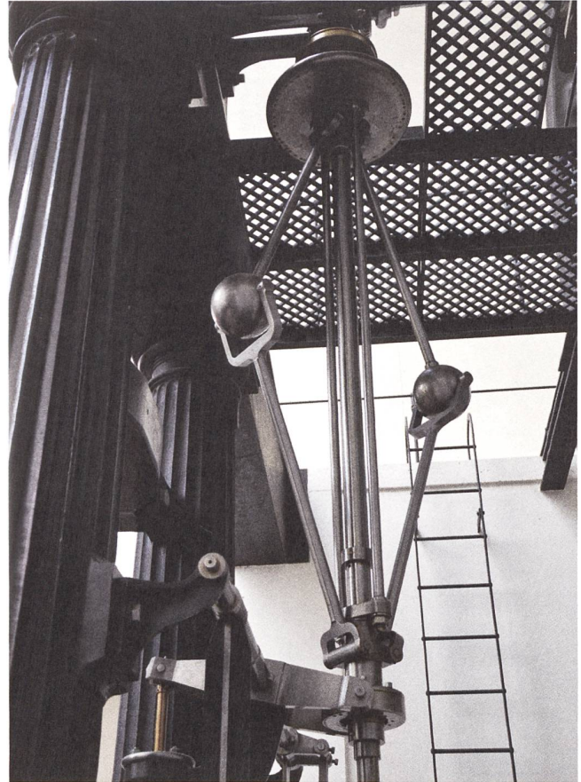
7b Detail of the engine's centrifugal governor controlling the precision tube valves.
