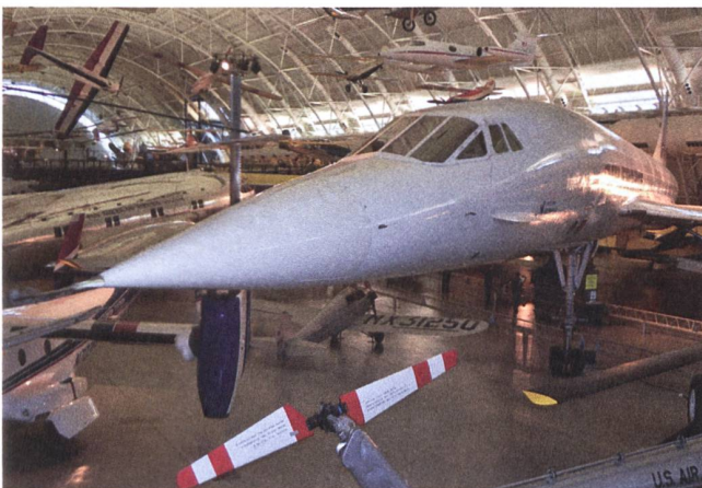
1 The raised nose of Concorde, essential for supersonic flight. It never malfunctioned.
