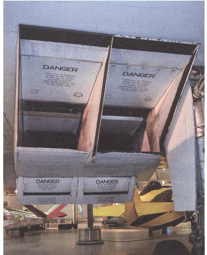
6 The right-side air intakes of Concorde F-BVFA on display at the Smithsonian National Air and Space Museum. The vane mechanism partially visible required several teams to assist in its design and testing.
