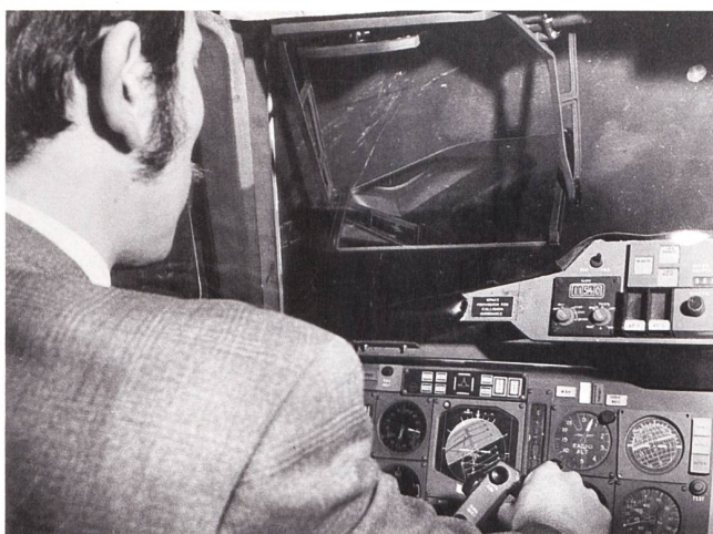
3 The proposed head-up display that airlines rejected. Airlines felt that commercial pilots would not be able to adjust to this kind of sophistication.
