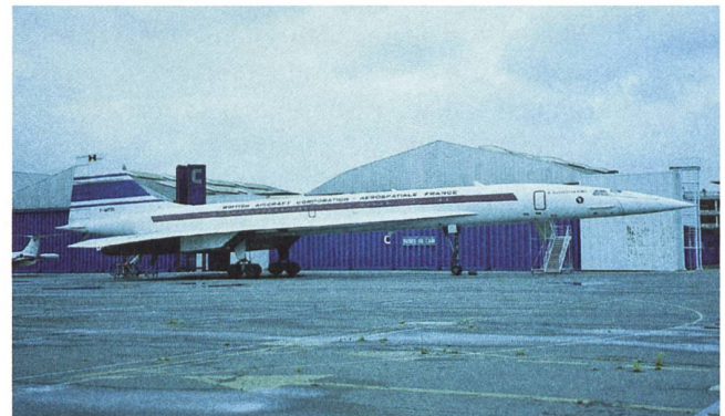
2 The first prototype at the Le Bourget museum near Paris with an opaque visor.
