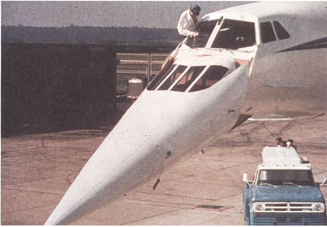
5 One of the pre-series aircraft during a visit to the United States shows its full 17.5 degree nose tilt. Commercial crew testing the plane complained that they felt disoriented not seeing the tip, and the droop was adjusted to 12 degrees instead.
