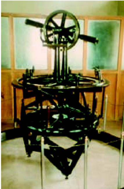
Fig. 7: The 36 inch diameter theodolite now at the Headquarters of the Survey of India in Dehra Dun.
