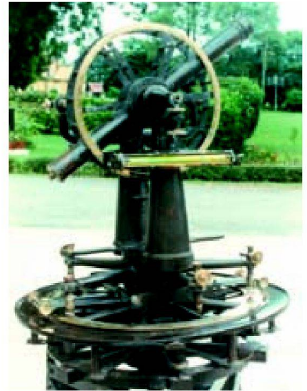
Fig. 6: 24 inch diameter theodolite used in India.
