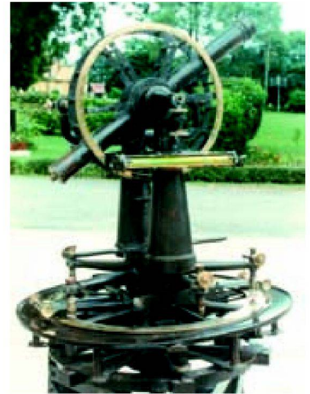
Fig. 6: 24 inch diameter theodolite used in India.
