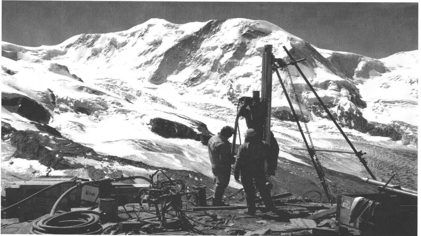
Photo 1: 100 m-deep borehole as part of the EU project PACE (Permafrost and Climate in Europe) on top of the Stockhorn (3420 m a.s.l.) at Zermatt, for long-term observation of the permafrost temperature in the rocks. In the background the frozen solid ice and cliff faces of the Lyskamm in the Monte Rosa Group.
