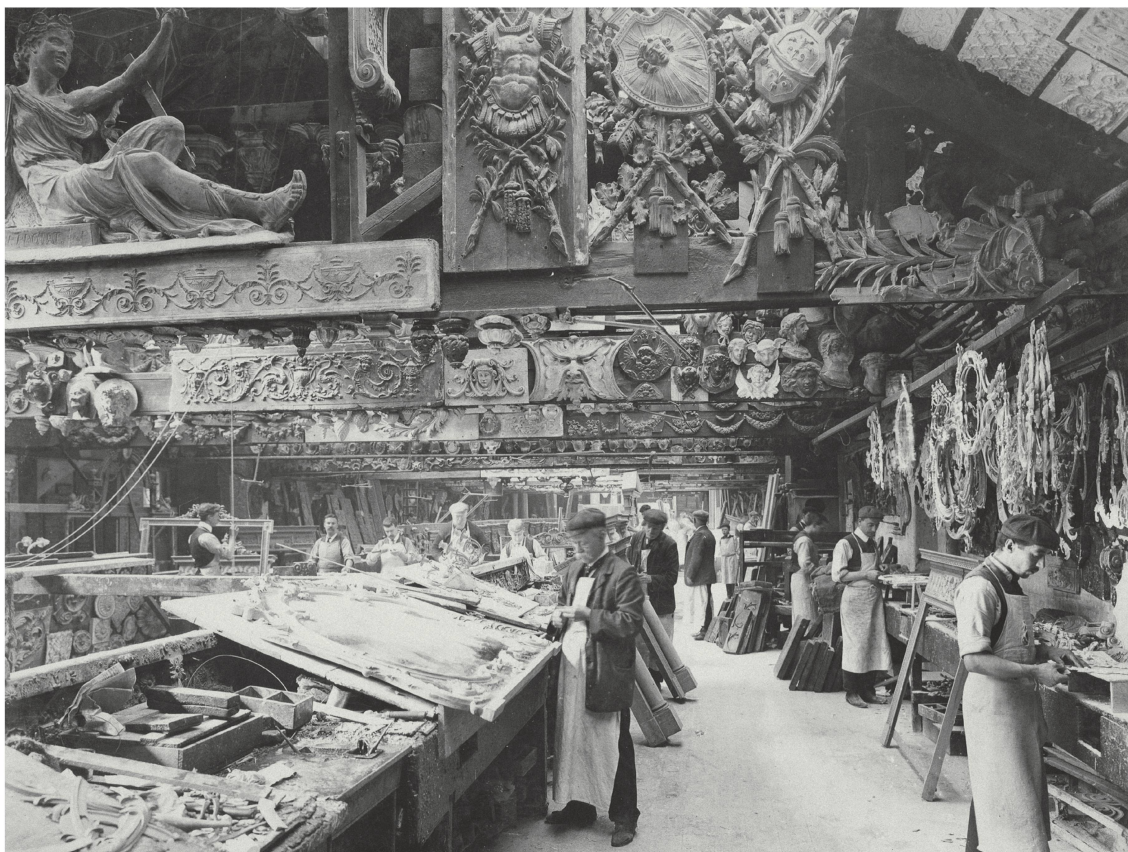
figs. 6 and 7 Workshops of George Jackson and Sons, n.d. (latter half of the nineteenth century). Two views of an ornament display room and workshop, showing workers drafting ornament designs and featuring press machinery for composition ornament Photographer: unknown Source: George Jackson Ltd., Company Archives
