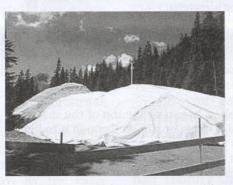
of snow into a seven-metre high pile. Half was covered with fleece and half with a 40cm layer of sawdust.
