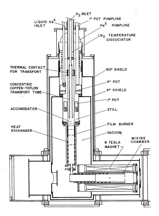
Fig. 1 The Michigan - MIT - CERN polarized proton jet
