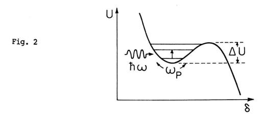
outside the well, the phase evolves with time and the junction is in its non-zero voltage state. The onset of the non-zero voltage state can easily be detected by measuring the voltage across the junction.
