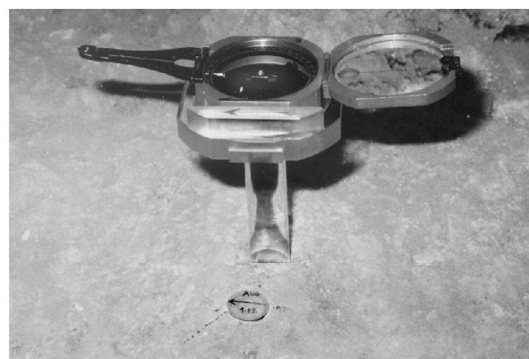
Fig. 3: Kaiseraugst, Liebrüti, tile kilns. Sampling of the floor of the large tile kiln using the glued-disc technique. Orientation of the specimen using a geologist's compass and a plastic distance piece.
