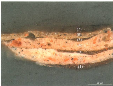
Fig. 11 Das Konzert : light microscope photograph of a cross-section of a sample from the flesh tint, left hand of the figure on the left. Brown glazes (1, 3, 5) alternate with opaque paint layers (2, 4, 6), followed by an application of varnish (7).
