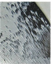
Fig. 8 Detail of a brushstroke of Syntonos paint made by reconstruction of the formulation patented in 1894. The paint displays a texture similar to that seen in Fig. 7, but as yet no craquelure.
