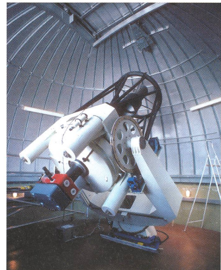
Fig. 10: The P3 photometer installed on the 1 m Lyon Ritchey-Chrétien telescope at Gornergrat.
