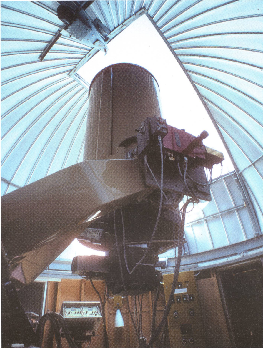
Fig. 16: The 70 cm Swiss Telescope at La Silla equipped with the P7 photometer.
