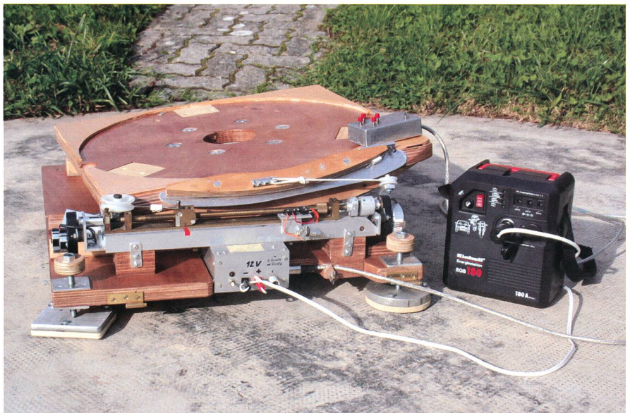
Figure 6: La Table Equatoriale du Dobson 425. (Photo: René Durussel)
