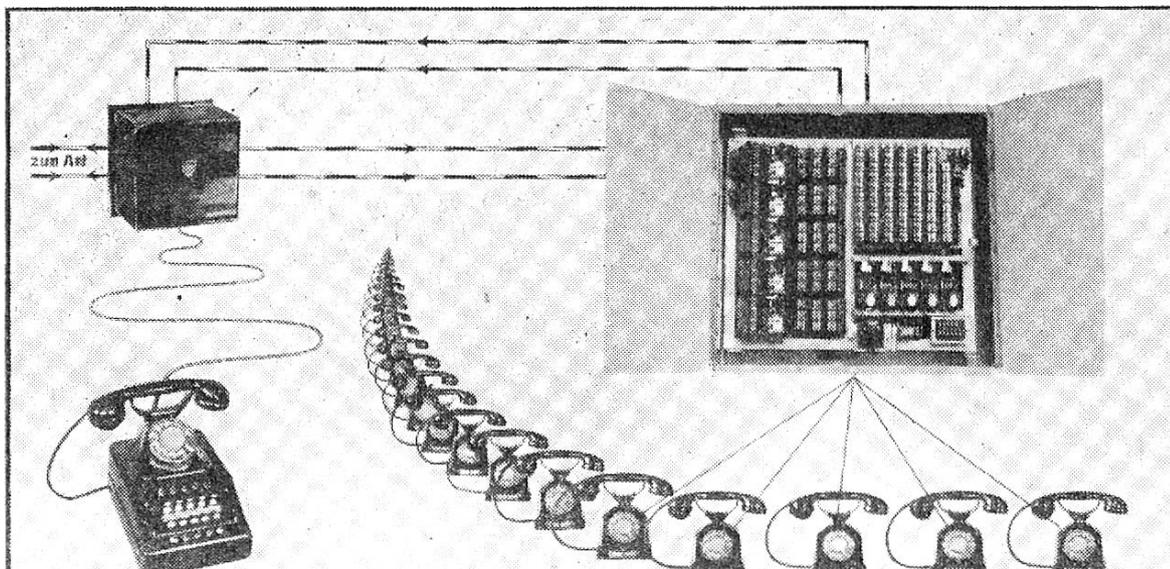
The diagram illustrates a telephone exchange system. On the left, a square box labeled 'zum Amt' (to the office) is connected to a switchboard. A series of lines connect the switchboard to a row of telephones. The telephones are arranged in a line, with the first one on the left and the last one on the right. The switchboard is a large cabinet with many vertical slots and a control panel. The telephones are of a classic design with a handset and a base.
