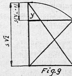
$$\begin{aligned} y:s &= s(\sqrt{2}-1) : s\sqrt{2} \\ y &= \frac{s(\sqrt{2}-1)}{\sqrt{2}} \\ &= \underline{\underline{\frac{2-\sqrt{2}}{2} s}} \end{aligned}$$
