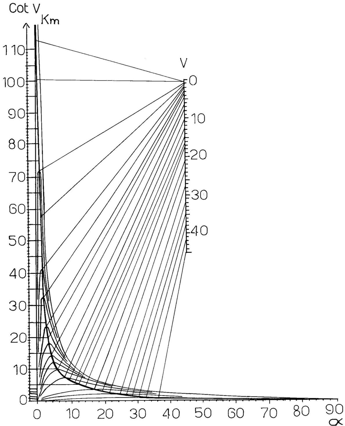
Fig. 2. Plane A.B.—O.N. It is seen that  $k$  increases from 0 at the symmetry axes to a maximum value in the A.B.—O.N. plane. In a considerable range of  $V$ -values  $k_{max} = \cot V$  so that  $V$  can be determined directly from this value even without the use of the graphs. This is true for  $2V$  values smaller than approx.  $45^\circ$ . In the straight portion near the symmetry axes  $\text{tg } \rho$  or  $k_{10}$  values can be also used to find  $2V$  (see fig. 4).
