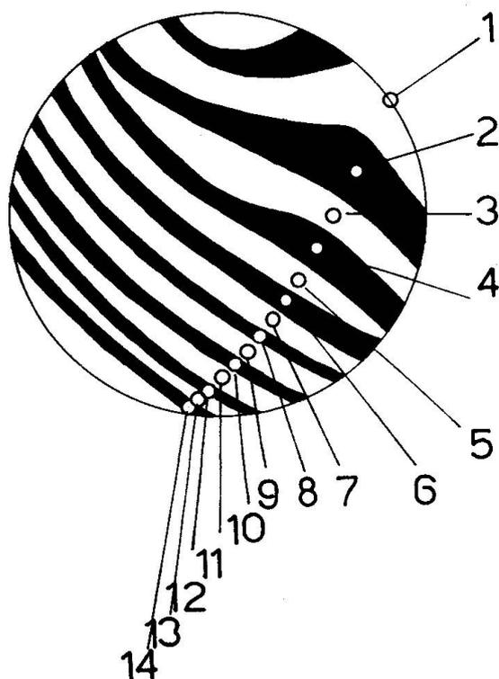
Fig. 6. Sketch of the photograph corresponding to the practical example. No symmetry axes and no O.A. are in the field. Objective UMK 50/0.60 (Leitz);  $\lambda = 480 \text{ m}\mu$ ;  $2V$  determined with the universal stage:  $44^\circ \pm 1$ . (Compare table 2 and fig. 7.)
