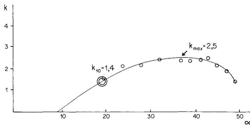
Fig. 8.  $k-\alpha$  curve for the practical example (see fig. 6 and table 2);  $\alpha$  = the angle of incidence referred to a certain direction of the interference figure contained in the symmetry plane. The size of the circle representing  $k_{10}$  gives an estimate of the error incurred in its determination.
