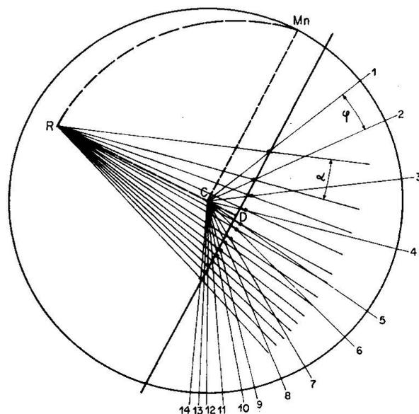
Fig. 7. Geometrical construction explained with the experimental method (p. 479).  $\overline{CM}_n$  = parallel to the gnomonic projection of the symmetry plane;  $\overline{CD}$  = perpendicular to this line;  $R$  = the angle point located on the prolongation of the perpendicular  $\overline{CD}$ ;  $\varphi$  azimuth of the directions of known retardation;  $\alpha$  = angle between these directions read on the tangent net fixed with  $R$  at its center.
