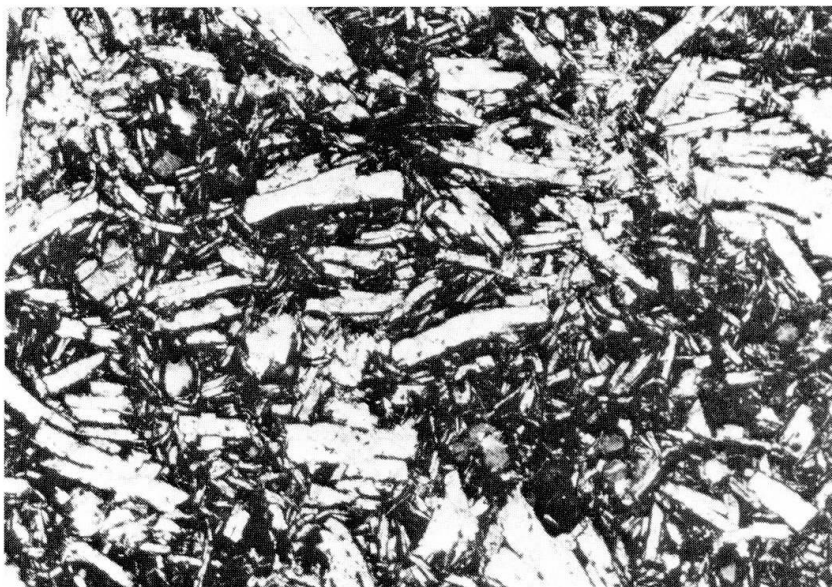
Fig. 3 Hematite spilite. Lath-shaped albites embedded in matrix with fine dispersion of hematite. Albite crystals often bent and oriented in fluidal texture. (length of base line, L = 3.27 mm, without analyser)
