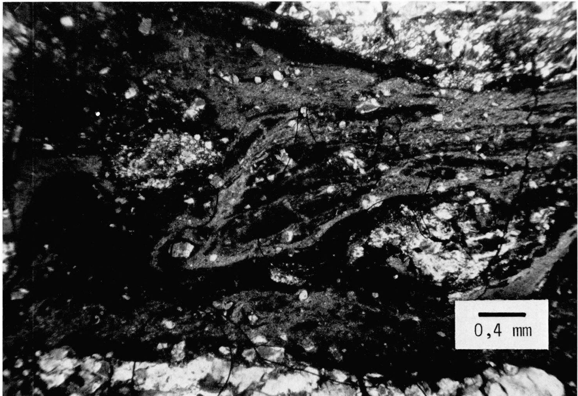
Fig. 6 Microscopic banding in the pseudotachylite matrix suggestive of flow-structures. Crossed nicols.
