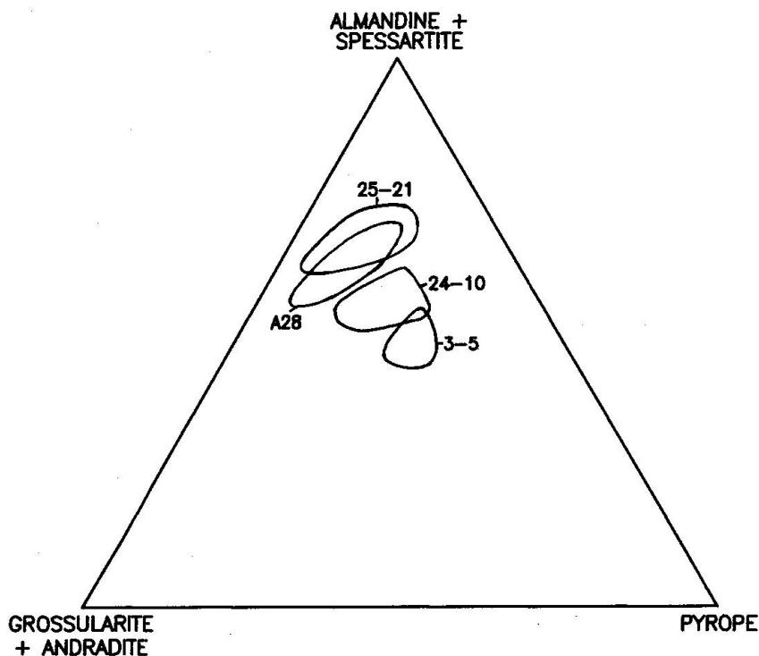
Fig. 5 Garnet compositions.  $\text{Fe}^{3+}$  has been calculated using charge balance and site saturation arguments.  $\text{CaO}$  decreases 2–3 wt% from the center towards the rims of the grains, whereas  $\text{MgO}$  and  $\text{FeO}$  increase by about the same amount.
