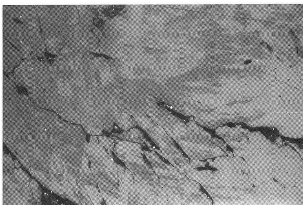
Fig. 3 Section of Fig. 2 but viewed under oil immersion. Oriented unidentifiable exsolutions with slightly lower reflectance become visible within the cervandonite-(Ce) matrix (maximum dimension of the photograph is approximately 100 \mu\text{m} ).
