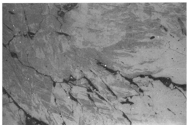
Fig. 3 Section of Fig. 2 but viewed under oil immersion. Oriented unidentified exsolutions with slightly lower reflectance become visible within the cervandonite-(Ce) matrix (maximum dimension of the photograph is approximately 100 \mu\text{m} ).
