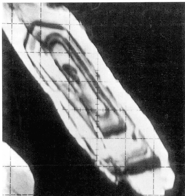
Fig. 3 Cathode-luminescence image of the grain shown in Fig. 1 (width ca. 60 \mu\text{m} ). Multiple euhedral zoning is indicated by the different C.L. response which is largely based on variable sums of trace and minor elements. Probably, this grain grew under variable P-T-X conditions during formation and ascent of the gabbroic protolith.
