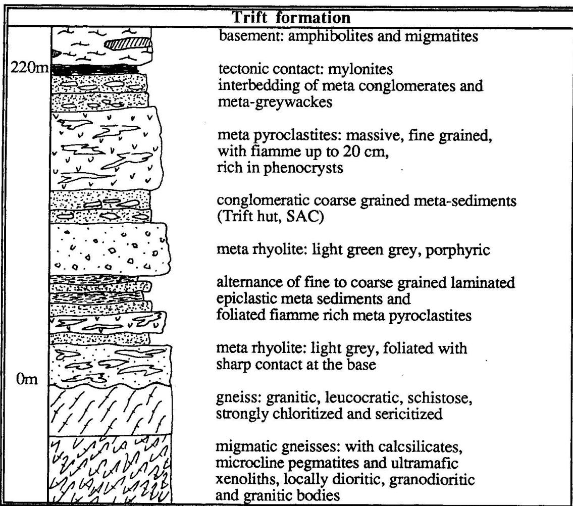
Fig. 3 Idealized section (profile) of the Trift formation modified after SCHENKER and ABRECHT (1987). Location of the base of this section: 671.500/170.075/2300.
