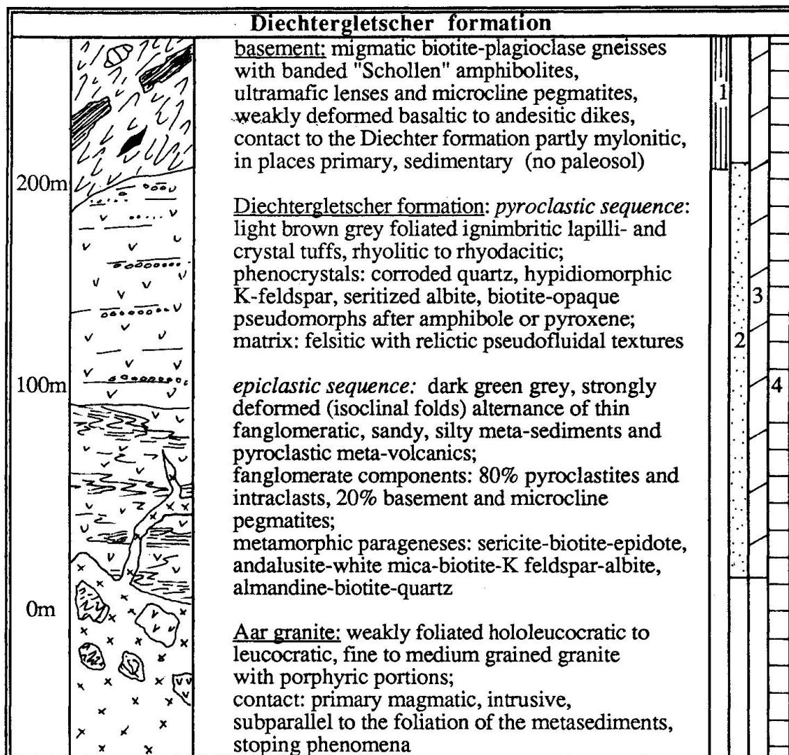
Fig. 4 Idealized cross section (N-S) of the Diechtersgletscher formation modified after SCHENKER and ABRECHT (1987). 1. pre-Variscan amphibolite-facies metamorphism with subsequent anatexis; 2. syn-volcanic hydrothermal alteration; 3. syn-granitic contact metamorphism; 4. Alpine greenschist facies metamorphism; Location of the base of this section: 669.175/166.950/2690.
