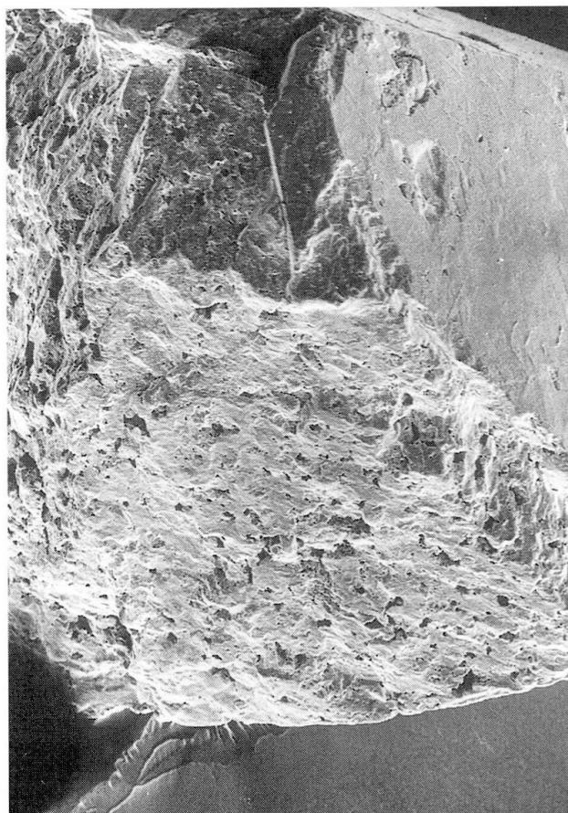
Fig. 3 Electron microscope image of a fragment of white milky zircon material, showing extensive porosity (sample KAW 128); magnification 360 \times .
