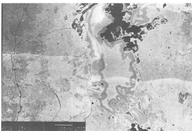
Fig. 7 SEM, BSE image, photomicrograph of sample 9: Penecontemporaneous braunite (br) and hollandite (hol) as principal manganese constituents, with pore-fill colloform hollandite and pyrolusite (pyr).
