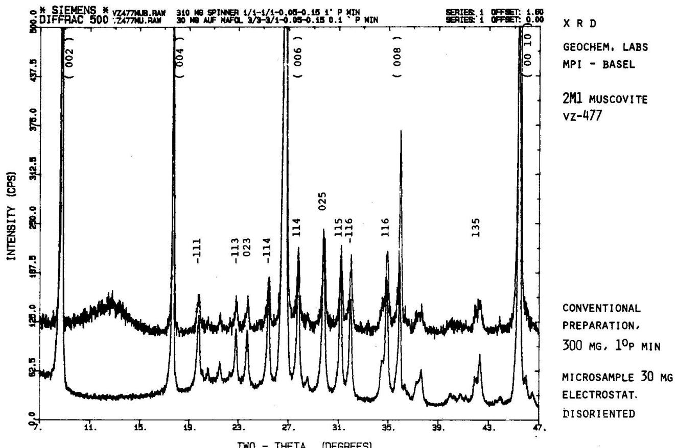
Fig. 1 X-ray diffraction pattern of powdered 2M1-muscovite (Vz 477): Comparison between conventional preparation (300 mg in sample cup) and electrostatically disoriented microspecimen (30 mg) on stretched foil. Non-basal reflections of the disoriented microsample display double net intensities.
