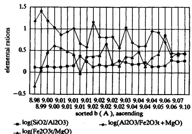
Fig. 5 Cell parameter  $b$  (XRD, experimental) and "phengite" content (XFA, experimental). Two elemental ratios are indicative, Si/Al connected with phengite content, and Al/Fe + Mg with ferrimuscovite and phengite content. Though a trendlike correlation between  $b$  and phengite content (XFA) exists, the interdependence is far too weak to be used for analytical purpose (i.e. phengite analysis by XRD).
