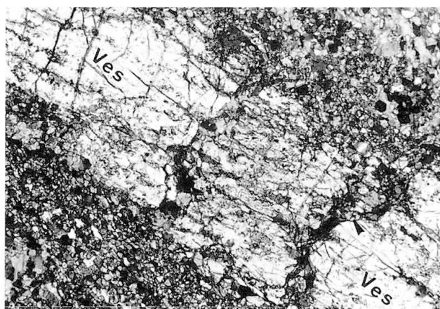
Fig. 13 Photomicrograph of fractured vesuvianite (Ves). Fractures contain diopside (indicated by the arrow). Long side of photograph is 5.2 mm. Crossed polarizers.
