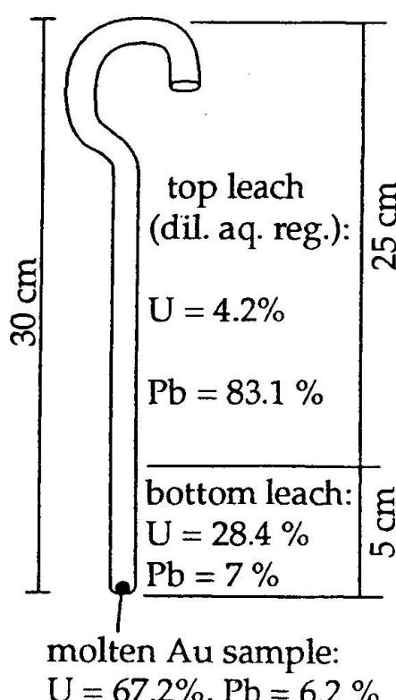
The results are given in figure 1. They demonstrate that  $\frac{1}{3}$  of total [U] and more than  $\frac{1}{10}$  of the [Pb] were lost from the Au upon melting. The accurate determination of [U] in an outgassed sample is only possible if the volatilized U is included in the calculations. As the percentage of U volatilization is probably a function of crucible temperature, it might be possible to get internally consistent, but too old, U-He ages by exactly repeating the outgassing procedure.
