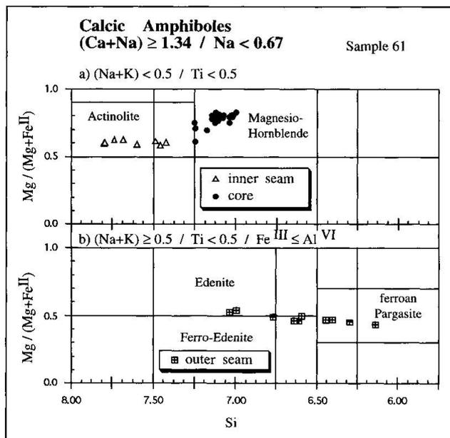
Fig. 10 Amphibole classification scheme after LEAKE (1978) used for zoned amphibole in metagabbro. 44 spot analyses of single, zoned amphibole grain in sample 61. Formula calculations according to ROBINSON et al. (1982, p. 6-9). Total cations exclusive of Na, K and Ca were normalized to 13,  $Fe_2O_3$  was then computed to obtain 23 oxygen / formula unit.
