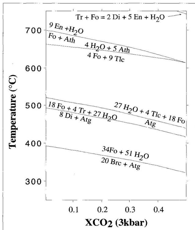
Fig. 13 T- $X_{CO_2}$ -diagram of the system CaO-MgO-SiO<sub>2</sub>-H<sub>2</sub>O, calculated with MacPTAX (LIEBERMAN, 1991) for phases in figure 12.
