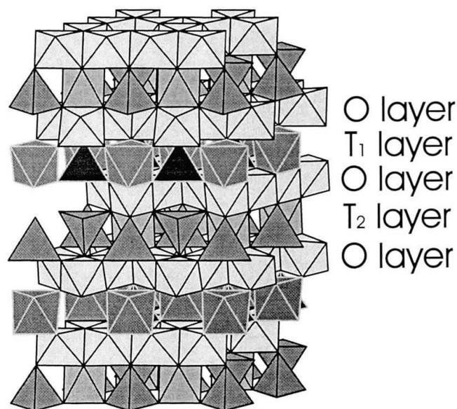
Fig. 1 Polyhedral representation of the zincohögbomite-8H structure. **O**-type octahedral layers are light gray with dark rims. **T<sub>2</sub>**-type spinel layers are dark gray with black rims and nolanite-like **T<sub>1</sub>** layers have light rims.
