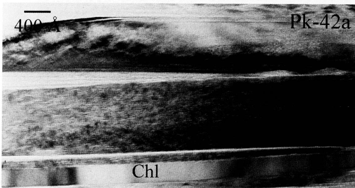
Fig. 7 Lattice-fringe image showing a detail of a chlorite-mica stack in which a defect-free chlorite packet of 20 layers is located within thick mica packets.
