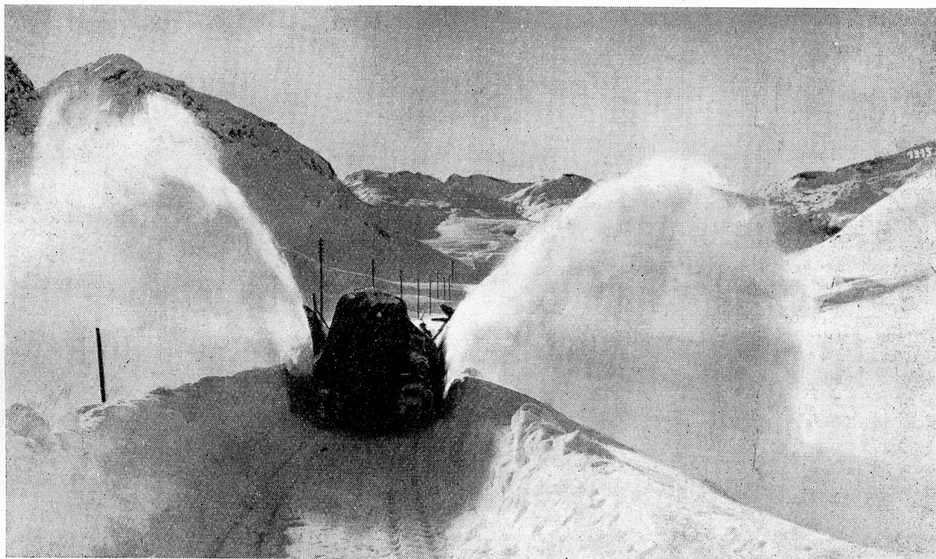
Clearing the Julier Pass by means of a Rotary Snow Plough of the Swiss General Post Office.
