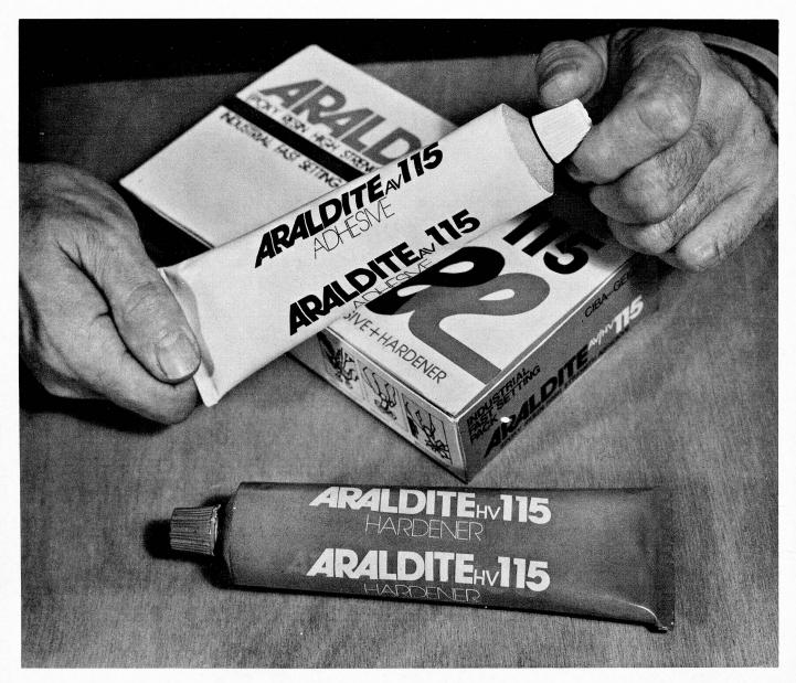
Araldite epoxy resin adhesive, in industrial-size packs, is now available as a quick-setting formulation known as Araldite 115. The packs comprise two large tubes from which equal amounts of resin and hardener can easily be dispensed and mixed together. The mixture remains usable, under average conditions, for about five minutes and hardens after about half-an-hour. Joints reach full strength within two hours. Distribution of this Swiss product from Ciba-Geigy is through engineering suppliers.
