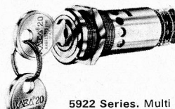
5922 Series. Multi position key actuated miniature rotary switch 0.3 amp at 220 Vac.
